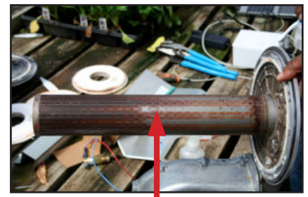
Burner & door assembly - prior to fiberboard installation
