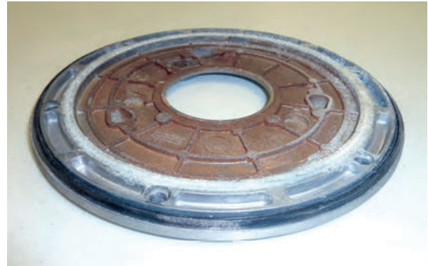
Damaged Burner Door
