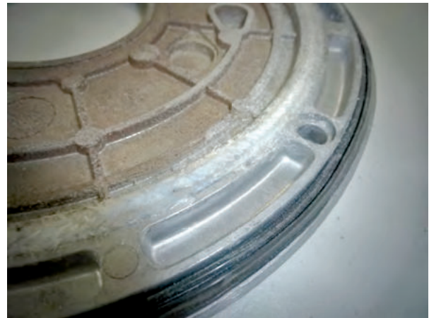
Damaged rope gasket—will not seal properly
